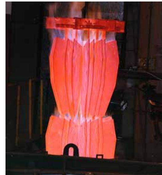
Kverneland 12 hours carburising process results in creating 2 steels in 1 sole mouldboard: flexible inside to absorb shocks and hard as a diamond on the outside for optimum wear resistance.
